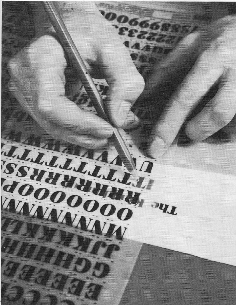
15 Using dry-transfer lettering. The backing sheet prevents accidental transfer of letters if placed between the lettering and album page. The dashes beneath the letters are used for alignment
